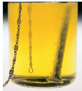
▲ FIGURE 1-3 A chemical property of zinc and gold: reaction with hydrochloric acid The zinc-plated (galvanized) nail reacts with hydrochloric acid, producing the bubbles of hydrogen gas seen on its surface. The gold bracelet is unaffected by hydrochloric acid. In this photograph, the zinc plating has been consumed, exposing the underlying iron nail. The reaction of iron with hydrochloric acid imparts some color to the acid solution.
